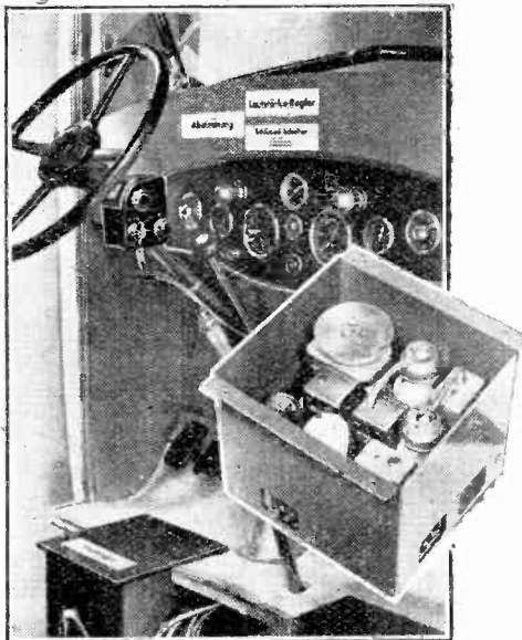
Telefunken motor-car receiver. Control box on the steering column: Inset: The four-valve superhet receiver.
