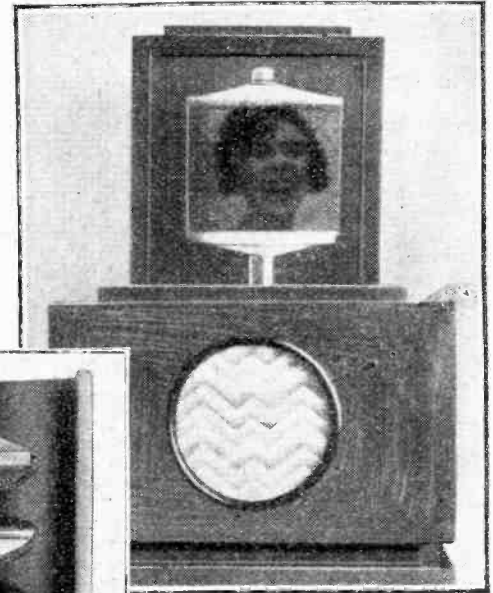
The Te-ka-de mirror screw television receiver and an enlarged view of the mirror screw and motor.
