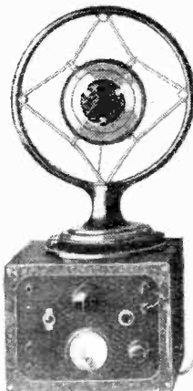
Ardente microphone and amplifier.
